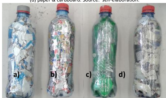
Figure 1. Eco-brick samples with single type fillers: (a) tetrapack; (b) metal; (c) PET; (d) paper & cardboard. Source: self-elaboration.
