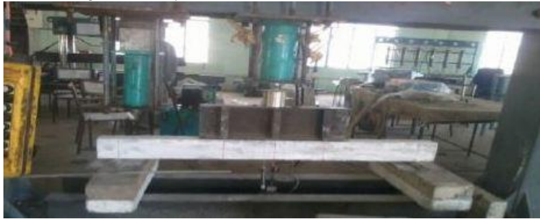
Figure 4. Test set up for reinforced concrete beam, Source: Self-Elaboration.
