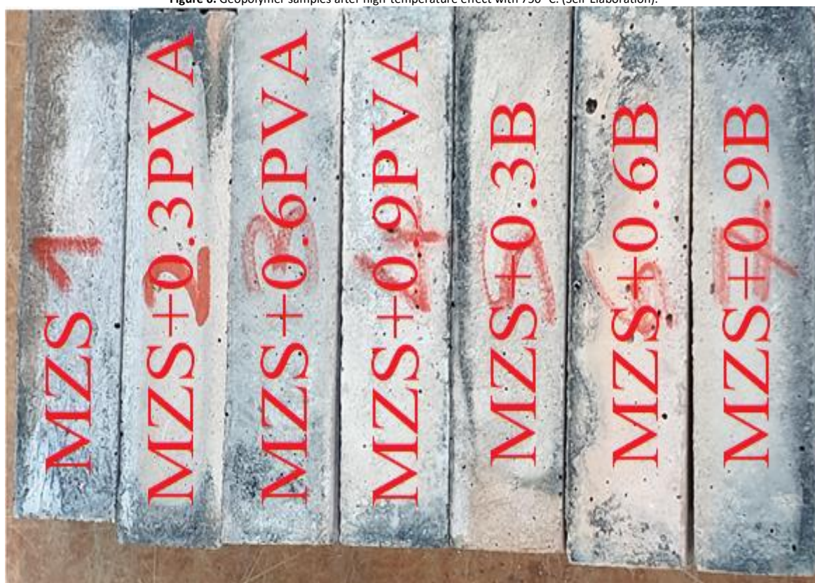
Figure 6. Geopolymer samples after high-temperature effect with 750 °C. (Self-Elaboration).
