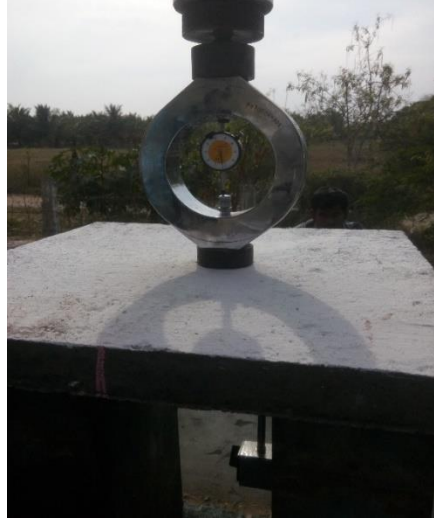
Figure 2. Typical slab during impact load loading. Source: Self-Elaboration.
