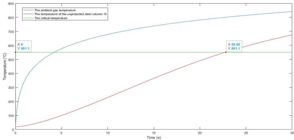
Figure 7. The time-temperature curves of the unprotected steel column with maximum values of cross-section.
