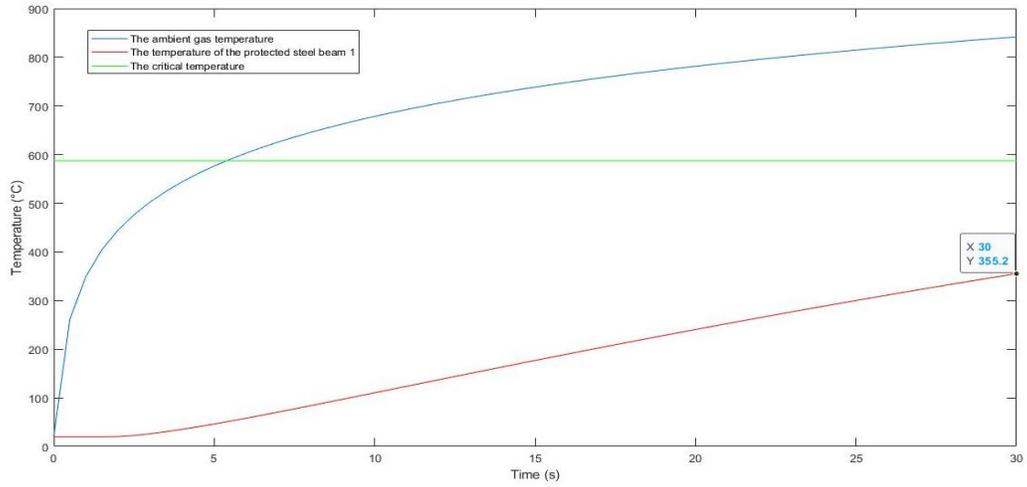
**Figure 8.** The time-temperature curves of the protected steel beam with optimal cross-section for case 2.
