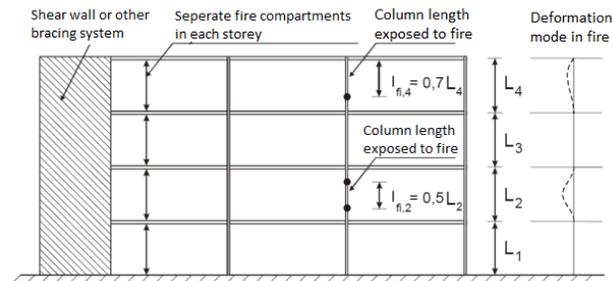
Figure 4. The buckling length of columns in case of fire.
