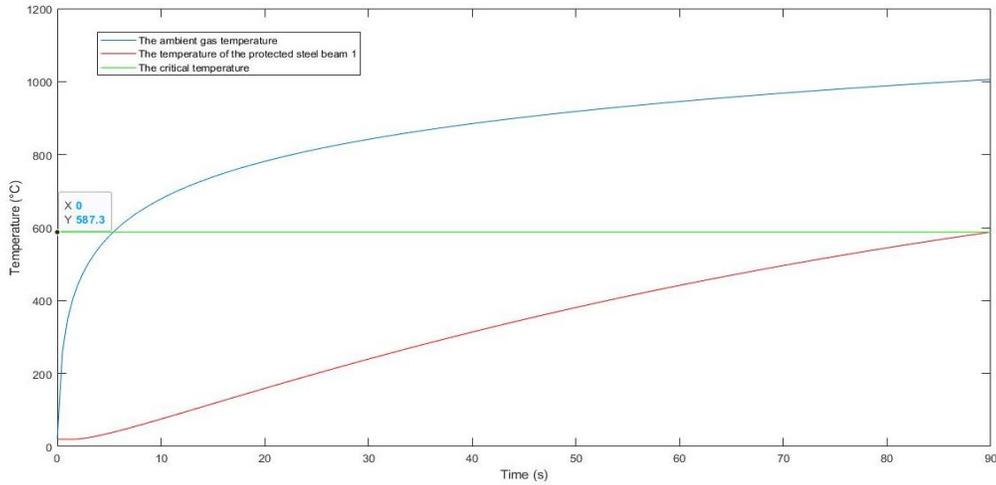
Figure 5. The time-temperature curves of the protected steel beam with optimal cross-sections for Case 5.
