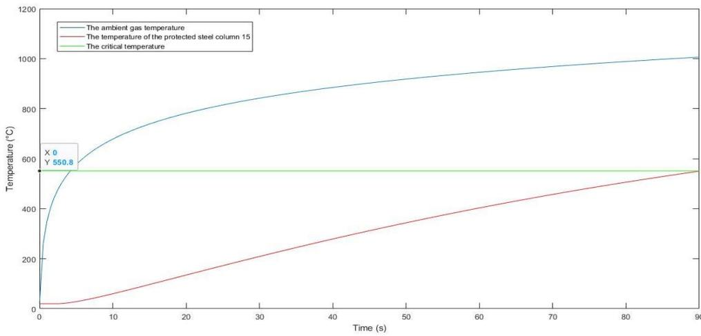
Figure 6. The time-temperature curves of the protected steel column with optimal cross-sections for case 6.
