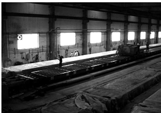
Figure 1. Sleepers factory. Long line process
