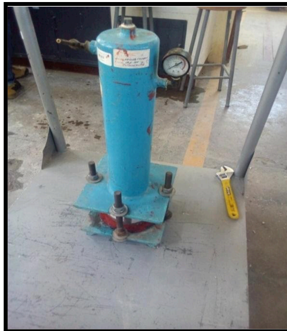
Figure 11. Permeability test for a resistance of 210 kg/cm 2 Source: own
