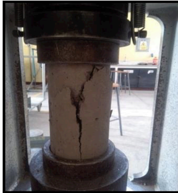
Figure 9. Compressive Strength Test Source: own
