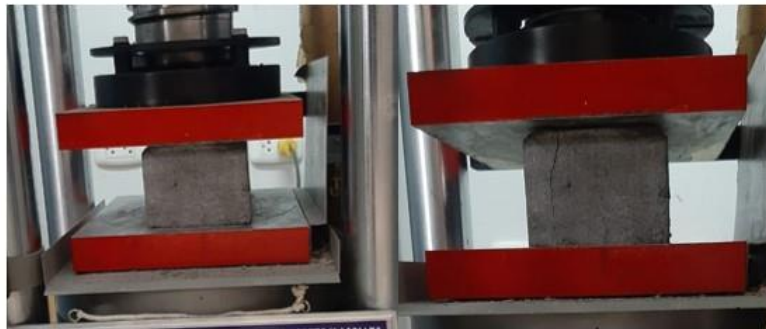
Figure 4. Compressive strength test and failure Source: Own source, 2021
