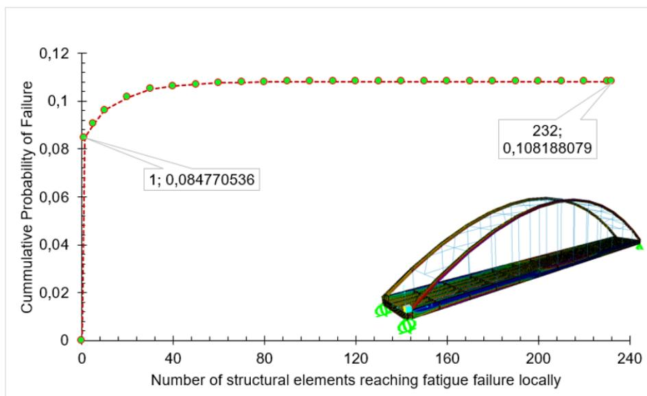
**Figure 23.** The theoretical probability of failure curve (fatigue vulnerability curve) for the Unete steel arch bridge as a function of the joint state of structural elements meeting fatigue failure
