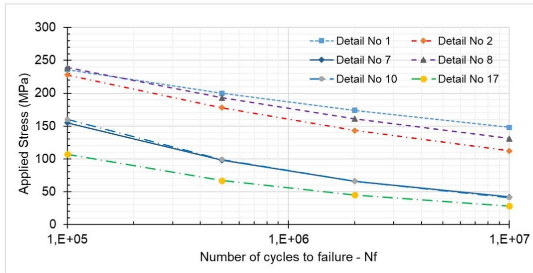
**Figure 5.** Fatigue S-N curves for uncorroded Steel for the structural elements fatigue details according to the reported data of (Ang and Munse, 1975)
