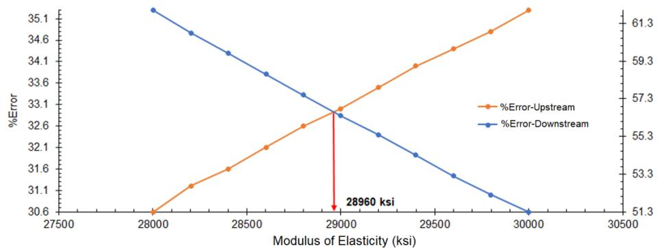
**Figure 14.** Systematic variation for the Unete steel bridge modulus of elasticity. Reported errors between the measured point of control vertical displacement and the simulated vertical displacement
