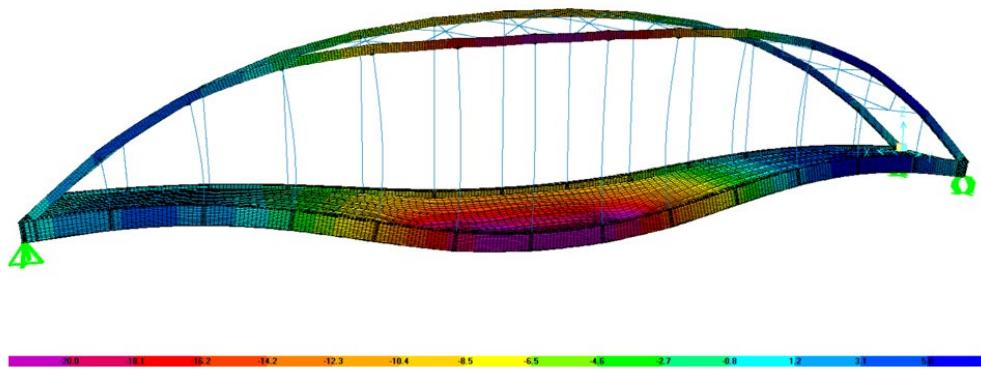
**Figure 15.** Eccentric vertical deformation of the finite element model for the Unete steel arch bridge. Loading case PC-1 (Units in mm)
