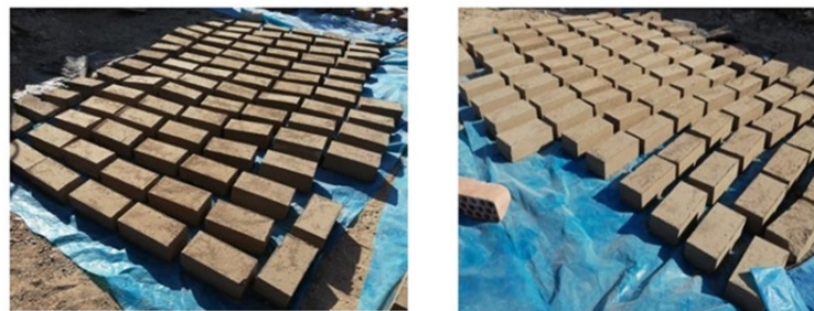
Figure 5. Drying process of the brick samples
