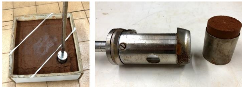
Figure 4. Extraction of a compacted soil sample to determine its moisture content by the oven drying method.
