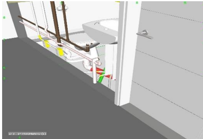
Figure 10. Interference of hydraulic pipes near electrical switchboards
