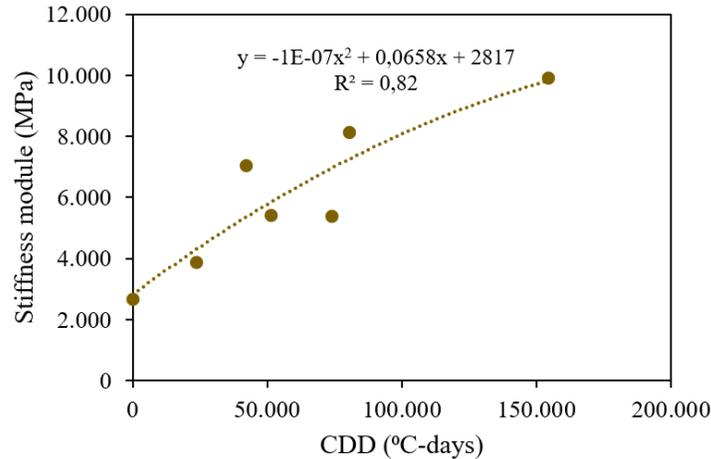
**Figure 5.** Variation of stiffness modules versus the CDD
