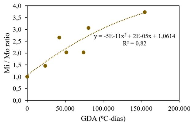
**Figure 6.** Variation of stiffness ratio versus the CDD
