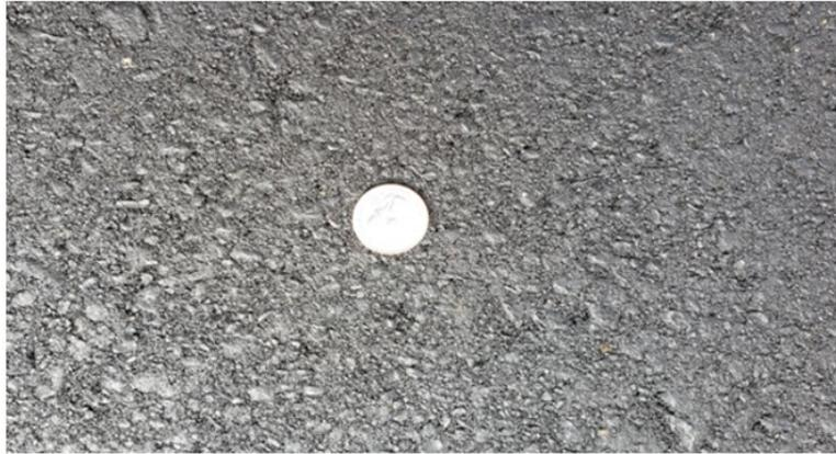
**Figure 7.** Surface damage for CDD=0 °C-days
