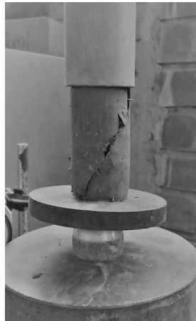
Figure 6. Unconfined compressive strength in treated soil
