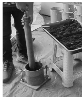
Figure 4. Compaction test with treated soil
