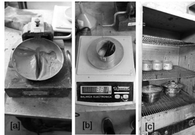
Figure 3. Treated soil (a) Liquid limit, (b) Plastic limit, (c) Moisture content
