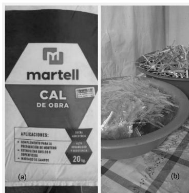
Figure 2. Additives, (a) Natural hydraulic lime, (b) plastic fibers and metallic fibers
