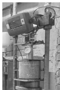
Figure 5. California bearing capacity in treated soil sample
